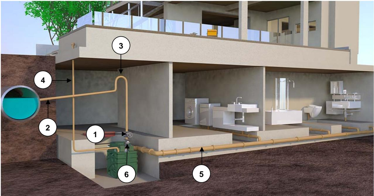
FEKABOX 110 are preassembled systems, ready for installation, requiring no adjustment, ideal for collecting and disposing of sewage and domestic waste water from basement rooms, situated below the level of the sewer network. In compliance with the accident-prevention regulations in force, the FEKABOX 110 cannot be used for conveying inflammable or explosive liquids, such as petrol, diesel fuel, combustible oils, solvents, etc.
