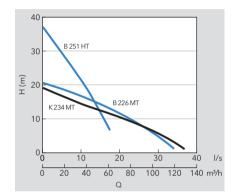
B = Wear-resistant impeller. K = Open impeller.
