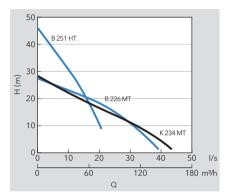
B = Wear-resistant impeller. K = Open impeller.
