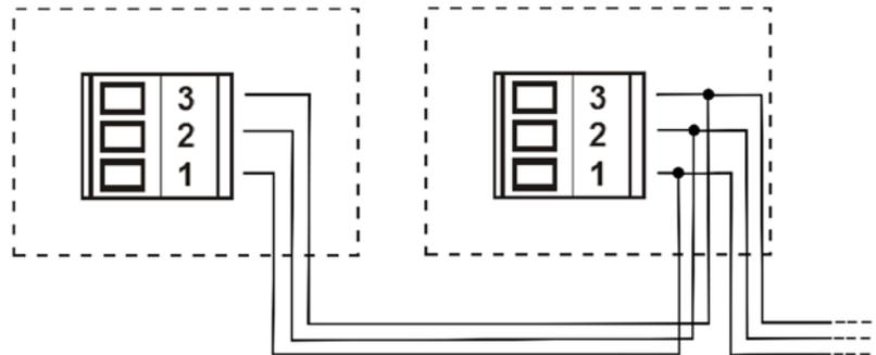
Figure 4: Connection of the multi-inverter communication
