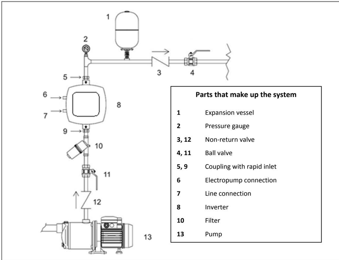
Figure 1: Hydraulic installation
