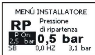
Figure 10: Setting the restart pressure
