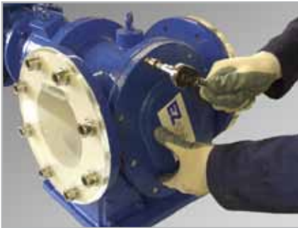
4. Loosen and remove shaft lock nuts
