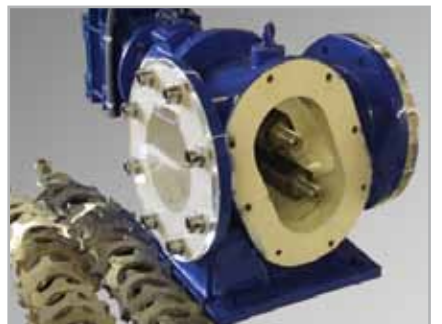
6. Inspect/replace cutters, spacers and shafts
