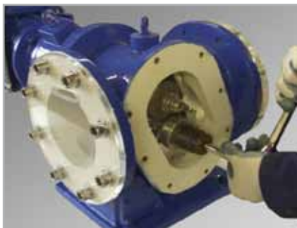
4. Loosen and remove shaft lock nuts
