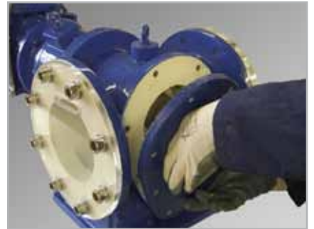
6. Inspect/replace cutters, spacers and shafts
