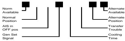
• After 5 minutes, transfer switch moves to normal source, and 'Cooling time' indicator appears.
