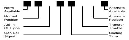
After the cooling time (5 minutes), the generator set signal is OFF and the engine stops.
