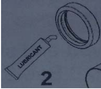
Gasket checking and lubrication
